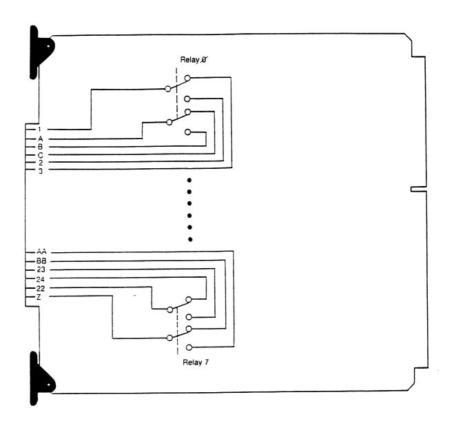
Figure 356-1: 53A-356 Card Block Diagram
